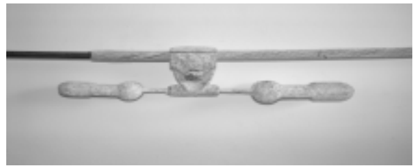
Figure 8. Test result after 1000 hours in the salt fog chamber
