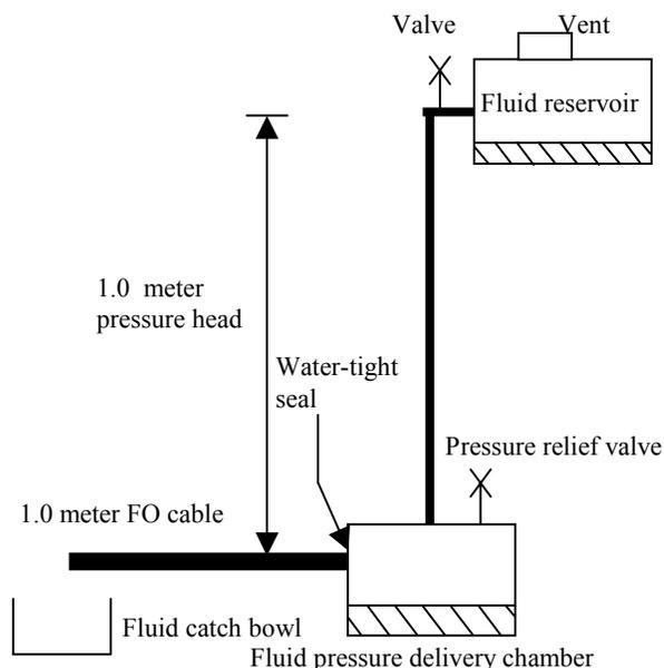
Figure 2. Longitudinal water penetration test set-up
