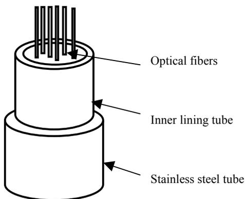
**Figure 4. Composite tube construction**
