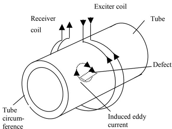
Figure 3. Physical principles of eddy current testing
